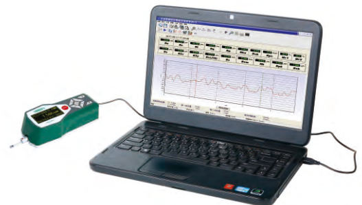
operate roughness tester by computers
